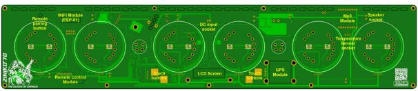
PCB is installed with components facing down, and once installed, you put acrylic sheet over it, plug in tubes and you're done. The diagram above shows location of controls and connectors on the PCB. While there are a lot of them, end user needs only the following:
